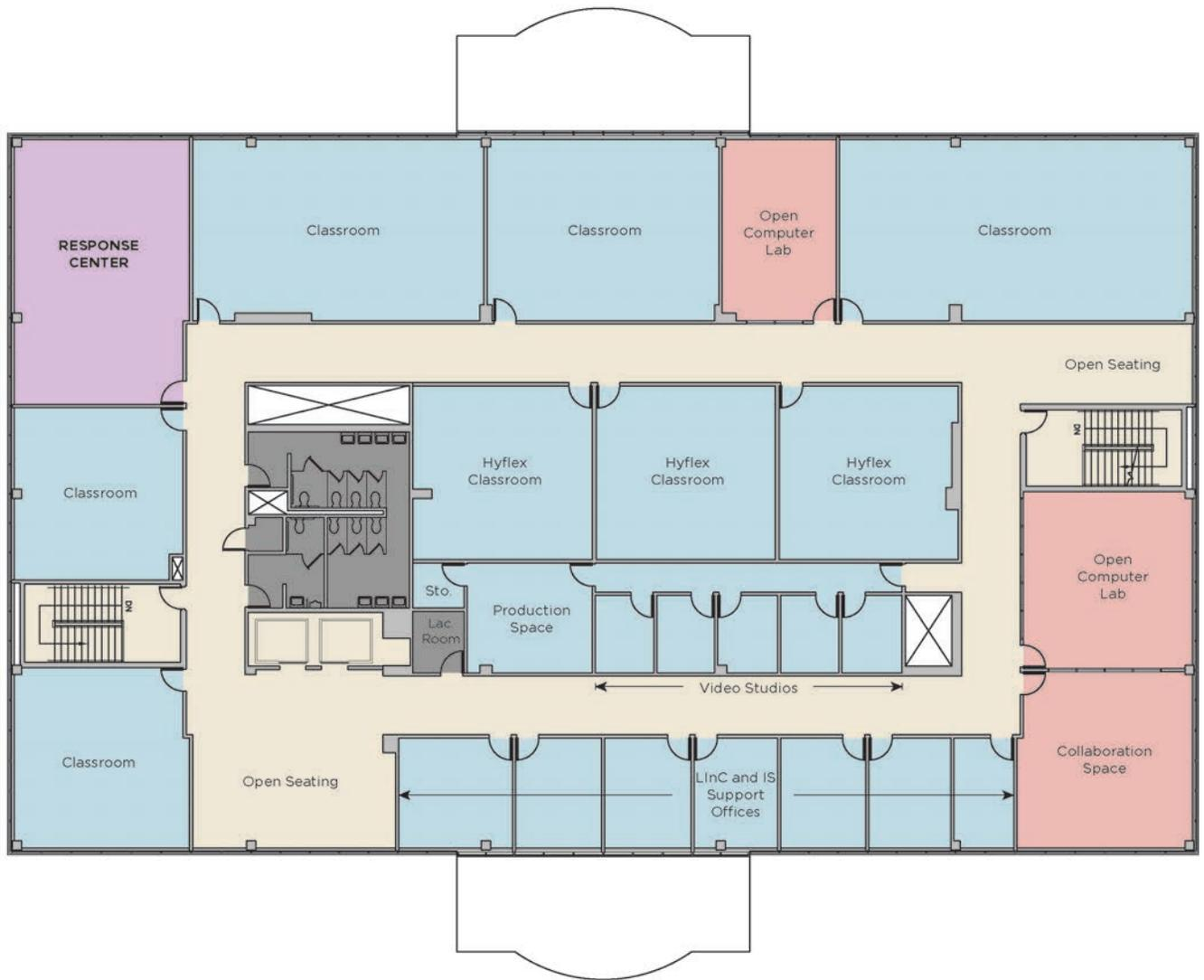
Figure 15: Conceptual Learning Innovation Center (LInC) Floor Plan
